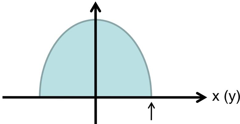
We define the beam with the edge of  $x = \text{sqrt}(\beta\epsilon) \times 2$  as  $1\sigma$  size beam
