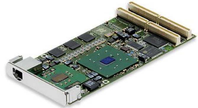
Photo of PSL09 w/ heat sink removed
