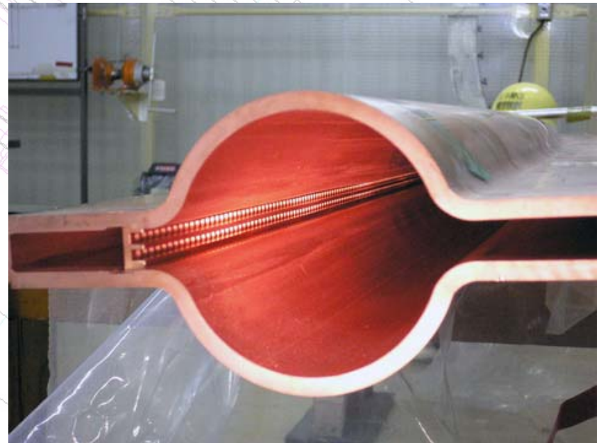
Slit for pump channel
