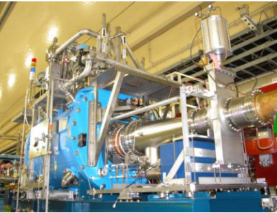
The superconducting cavities will be upgraded to absorb more higher-order mode power up to 50 kW.
