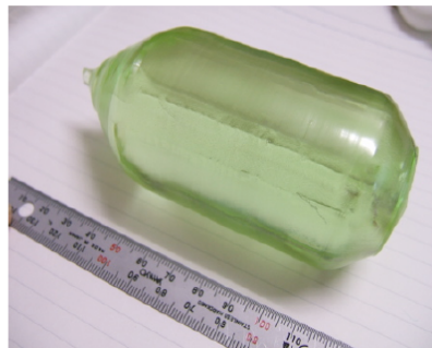
Crystal with Pr doping in 0.25 atomic%. 2in. diameter ingot
